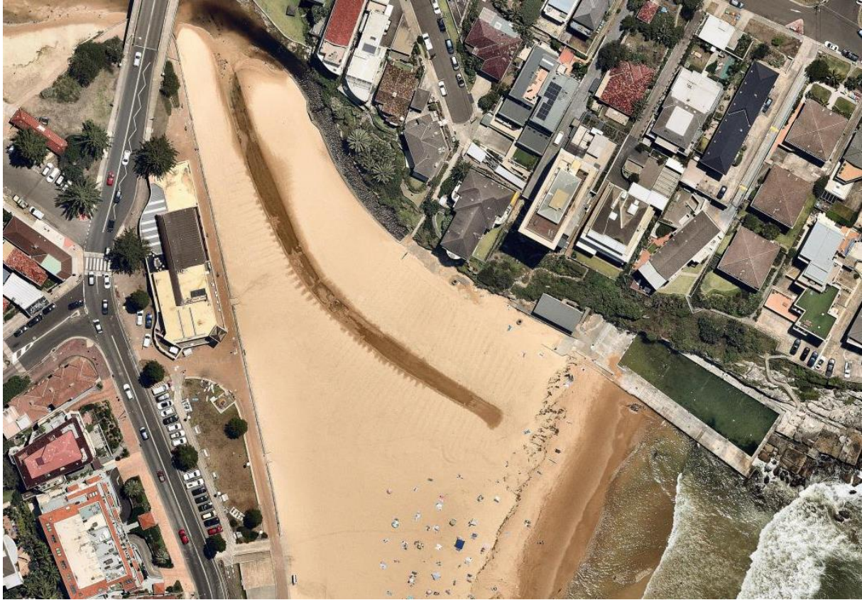
A.16: Channel across the beach used for flood mitigation (21/01/2021) (source: Nearmap)
